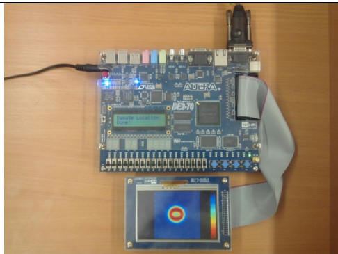
Figure 6(a): System based on FPGA Cyclone2 EP2C70.
